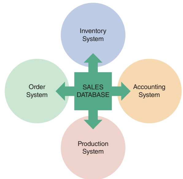
FIGURE 9-6 In this example, a sales database can support four separate business systems.
