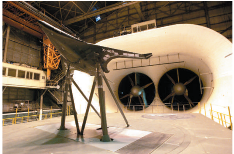
FIGURE 7-26 Wind tunnel testing is a typical example of prototyping.
