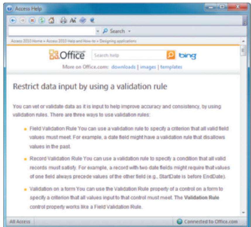
FIGURE 8-35 Validation rules can improve data quality by requiring the input to meet specific requirements or conditions.
