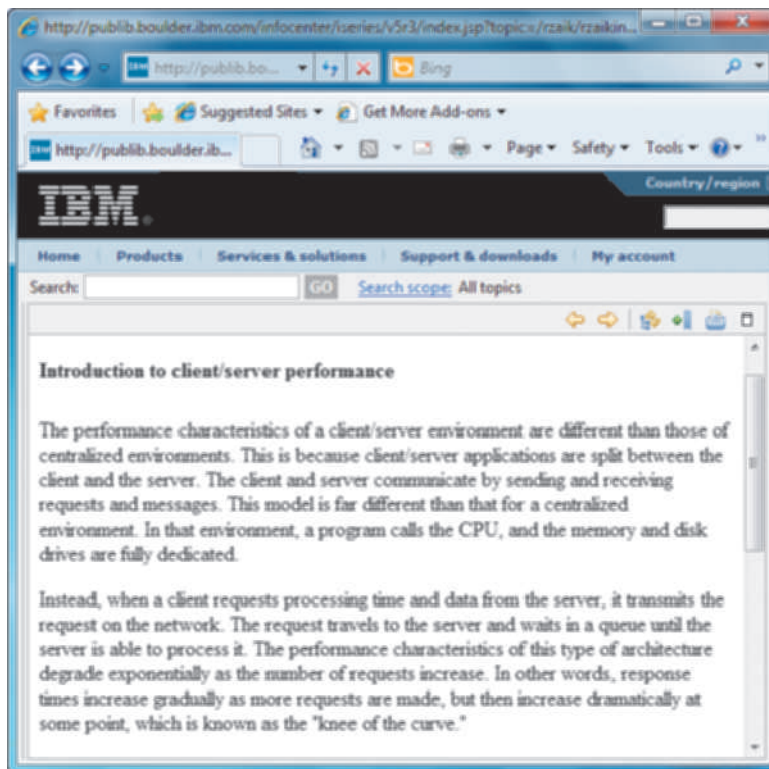
FIGURE 10-19 According to IBM, client/server response times increase gradually, and then rise dramatically when the system nears its capacity. That point is referred to as the knee of the curve .
