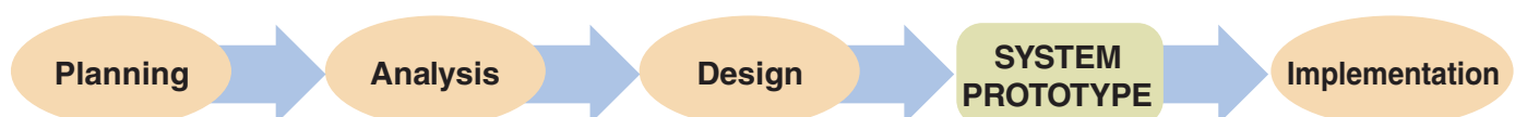
FIGURE 7-27 The end product of system prototyping is a working model of the information system, ready for implementation.
