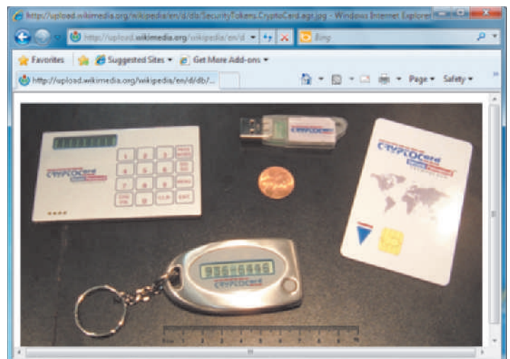
FIGURE 12-37 Security tokens, which come in various forms, can provide an additional level of security.
