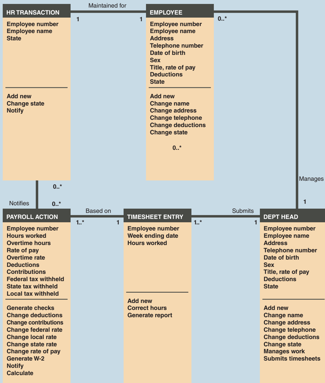
FIGURE 6-39 The GENERATE WEEKLY PAYROLL class diagram includes five classes and various types of relationships among the classes.
