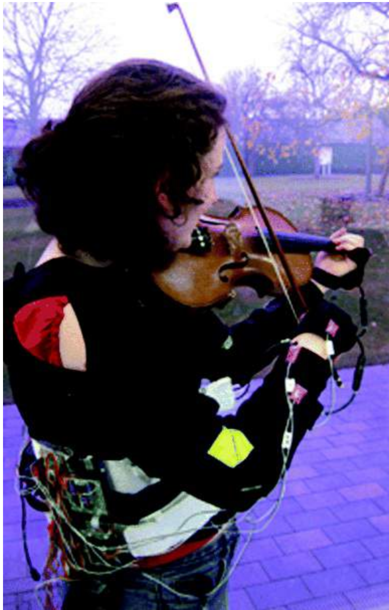
Figure 6.26 The MusicJacket prototype with embedded actuators that nudge the player
