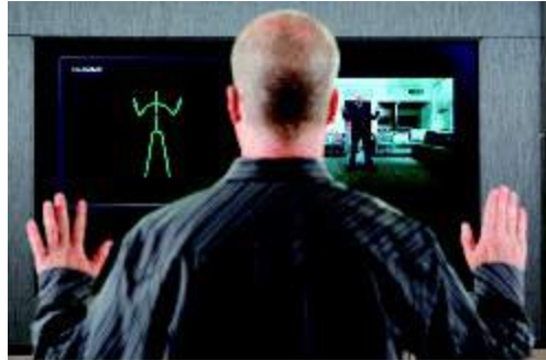
Figure 6.24 Microsoft's Xbox Kinect comprising an RGB camera for facial recognition plus video capturing, a depth sensor (an infrared projector paired with a monochrome camera) for movement tracking, and downward-facing mics for voice recognition
