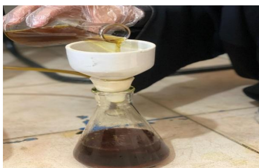
Figure(3.2) Filtration proces
